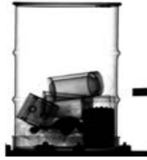
Figure 2: The container in the bottom right corner of this image appears to contain dense granules.
