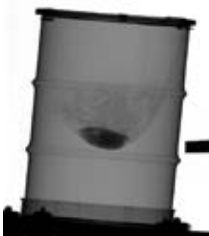
Figure 5: This drum contains dust in a PVC bag.
