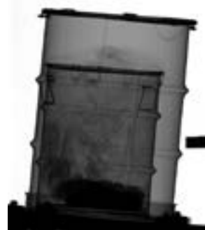
Figure 6: This inner drum potentially contains dust with rubble at the bottom.
